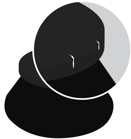
Cyclical stretching and relaxing of the rotor alloy causes microscopic changes in its structure, eventually leading to cracks and failure.
